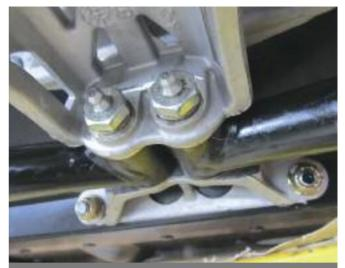
New lower A-arm bushing kit installed, ready for grease.
