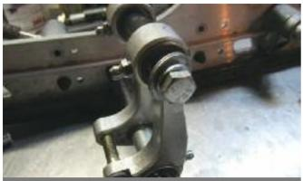
MSK-03-1 Rocker Arm Bushing Kit adds new, wider bushings as well as grease fittings to both pivot points. This is the linkage between the centre and rear shock. Free movement is important
