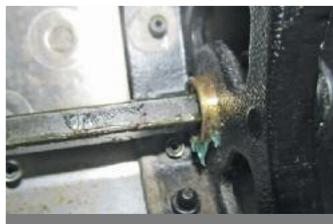
MSK07 kit adds an additional bushing for increased support and reduced freeplay.
