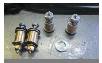
MSK02-1 Greasable Swing Arm Bushing Kit ready to install on the rear suspension's front arm.
