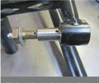
MSK01 Greasable Control Arm Kit. Note the ports for the grease to travel through the bolt to each pivot point.
